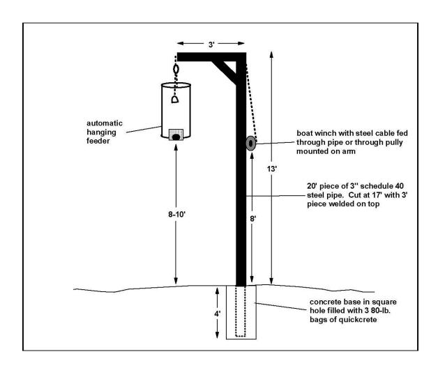
Figure 1. Diagram of how to hang a wildlife feeder out of the reach of bears.
